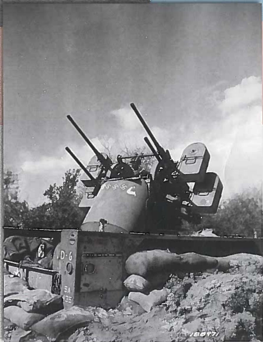
The M45 Multiple Caliber .50 Machine-Gun Mount entered service in 1942 and equipped the Army's antiaircraft artillery-automatic weapons (AAA-AW) battalions. Its four M2 .50 caliber machine guns made it an effective weapon against low-flying enemy aircraft. It was also devastating against ground targets and earned the nicknames "meat chopper" and "kraut mower." This example served with the 435th AAA-AW Battalion. (National Archives)
