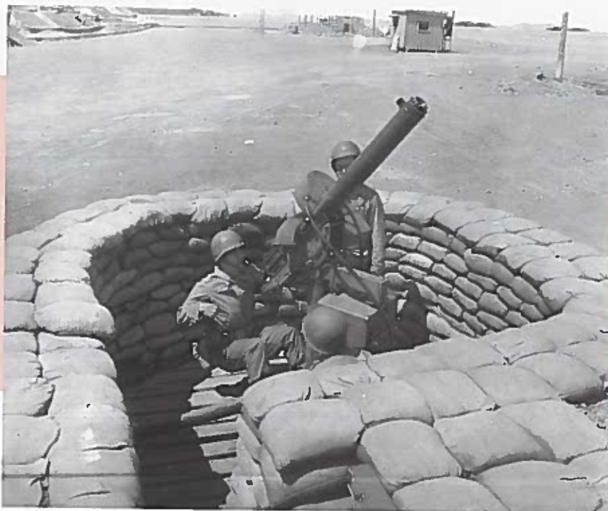
The water-cooled M2 .50 caliber (shown here) and M4 37mm gun served as the Army's standard AAA weapons against low-flying aircraft during the early years of the U.S. involvement in World War II. (National Archives)
